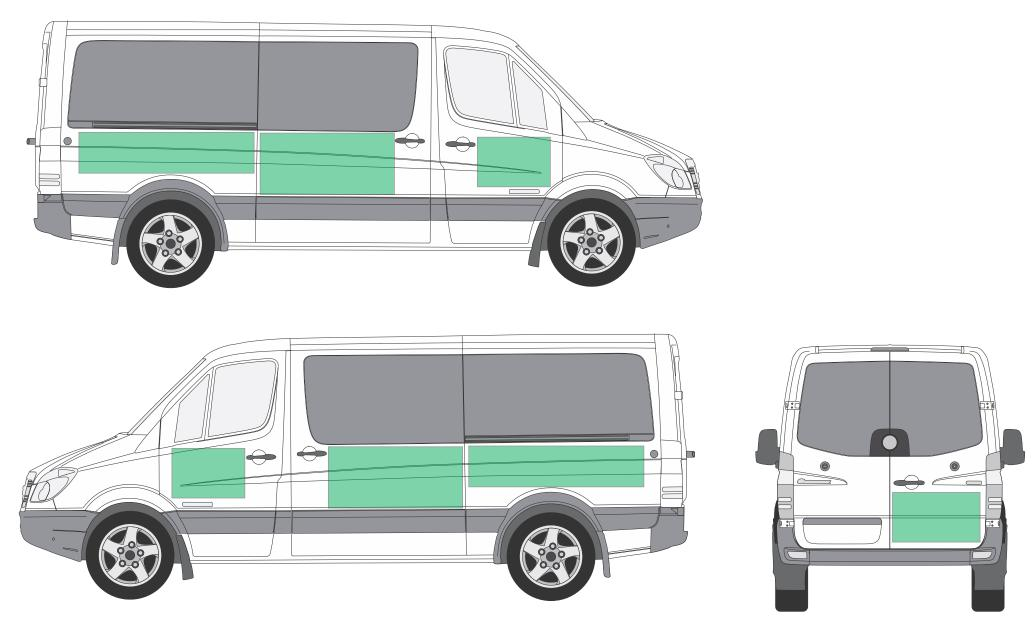
MercV\_015 Dodge Sprinter Window - Short (I44"Wheelbase) Standard Roof (65")
