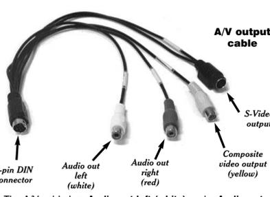
3. The **A/V** cable has **Audio out left (white)** and a **Audio out right (red)** jack. Connect these to the audio input jacks on your TV set (not supplied).
