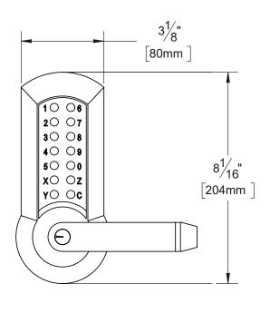
New Door Prep: 2 1/8" Cross Bore, 1" Edge Bore, 4 of 3/8" Through Bolt Holes
