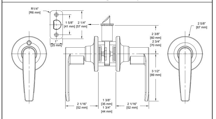
Door Prep: Cross Bore 2 1/8+, Edge Bore 1+, Mortise Latch Face 1+x 2 1/4+, Optional Drive In Latch 1" Diameter Drilled Hole
