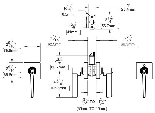
Door Prep: Cross Bore 2 1/8", Edge Bore 1", Mortise Latch Face 1" x 2 1/4", Optional Drive In Latch 1" Diameter Drilled Hole
