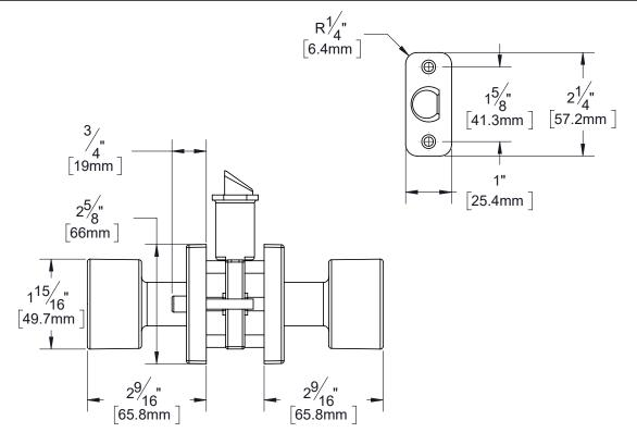
Door Prep: Cross Bore 2 1/8+, Edge Bore 1+, Mortise Latch Face 1+x 2 1/4+, Optional Drive In Latch 1" Diameter Drilled Hole Latches: Ships With Mortise Latch As Shown Above. Optional Drive In Or UL10C Fire Rated Latches Available
