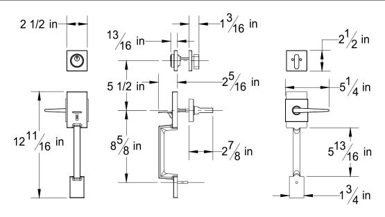
Door Prep: Cross Bore 2 1/8", Center To Center 5 1/2", Edge Bore 1", Mortise Latch Face 1" X 2 1/4" X 1/4" Radius,
