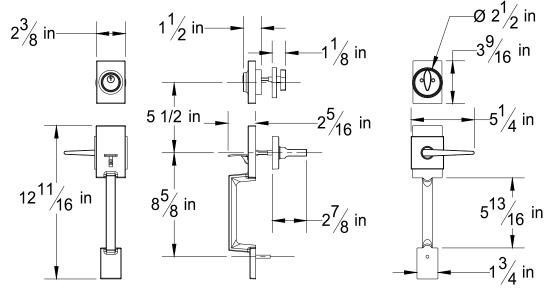
Door Preparation: Cross Bore 2 1/8", Center To Center 5 1/2", Edge Bore 1", Mortise Latch Face 1" X 2 1/4" X 1/4" Radius, Optional Drive In Latches Require 1" Diameter Edge Bores
