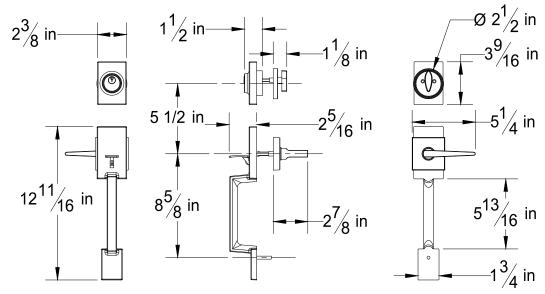
Door Preparation: Cross Bore 2 1/8", Center To Center 5 1/2", Edge Bore 1", Mortise Latch Face 1" X 2 1/4" X 1/4" Radius, Optional Drive In Latches Require 1" Diameter Edge Bores
