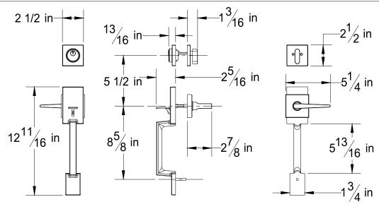
Door Prep: Cross Bore 2 1/8", Center To Center 5 1/2", Edge Bore 1", Mortise Latch Face 1" X 2 1/4" X 1/4" Radius,
