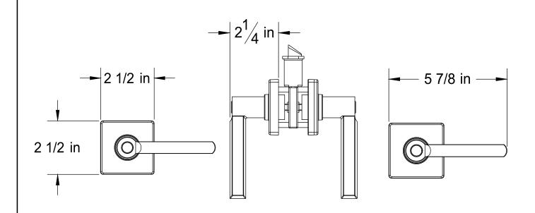
Door Prep: Cross Bore 2 1/8+, Edge Bore 1+, Mortise Latch Face 1+x 2 1/4+, Optional Drive In Latch 1" Diameter Drilled Hole
