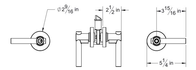
Door Preparation: Cross Bore 2 1/8", Edge Bore 1", Mortise Latch Face 1" X 2 1/4", Optional Drive
