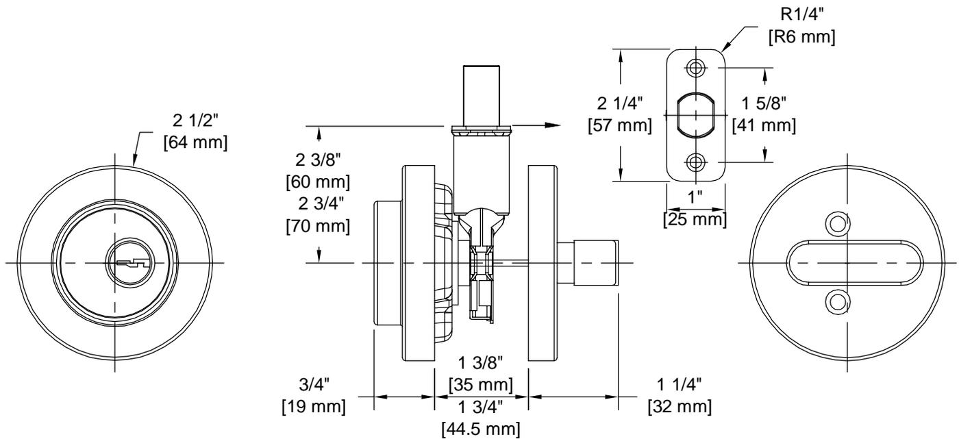
**Door Prep:** Cross Bore 2 1/8+, Edge Bore 1+, Mortise Latch Face 1+x 2 1/4+, Optional Drive In Latch 1" Diameter Drilled Hole
