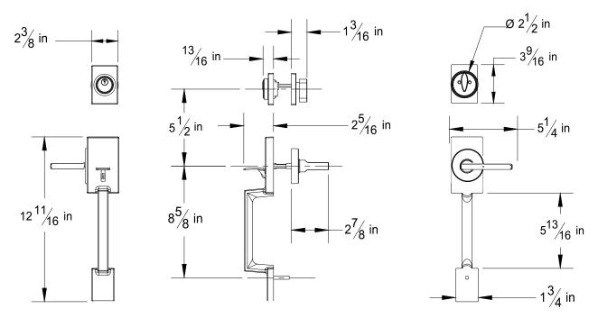
Door Prep: Cross Bore 2 1/8", Center To Center 5 1/2", Edge Bore 1", Mortise Latch Face 1" X 2 1/4" X 1/4" Radius, Optional
