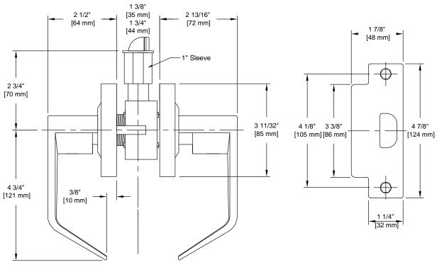
Door Prep: Cross Bore 2 1/8+, Edge Bore 1+, Latch Face 1 1/8+x 2 1/4+
