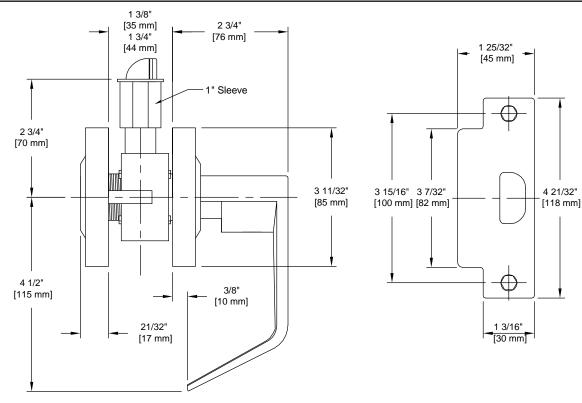
Door Prep: Cross Bore 2 1/8+, Edge Bore 1+, Latch Face 1 1/8+x 2 1/4+
