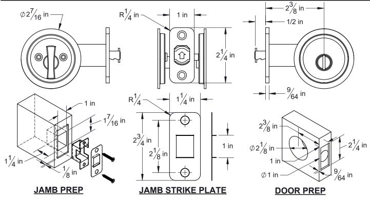
Door Preparation: Cross Bore 2 1/8", Edge Bore 1", Mortise Latch Face 1" X 2 1/4" Radius Corners
