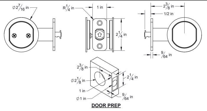
Door Preparation: Cross Bore 2 1/8", Edge Bore 1", Mortise Latch Face 1" X 2 1/4" Radius Corners
