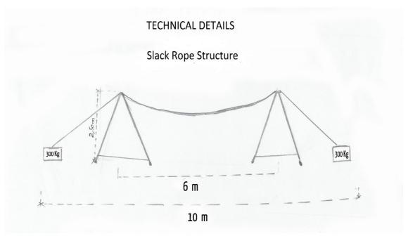
The "A" Structure is already build and it's necessary two points to attach on the ground or on the wall. the point to attach need to hold **300 Kg**.
