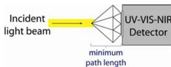
**Transmission absorption spectra** in the UV to near-IR range (250-1000 nm) were collected using a Hitachi U4001 spectrometer (2.0 nm slit, 1.0 nm data interval, and 120 nm/min scan speed). Unless otherwise noted, an unpolarized light beam was focused on the culet area of the optically unoriented sample.
