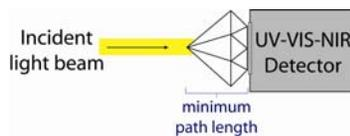
Visible Absorption | min. path length: 9.5 mm
