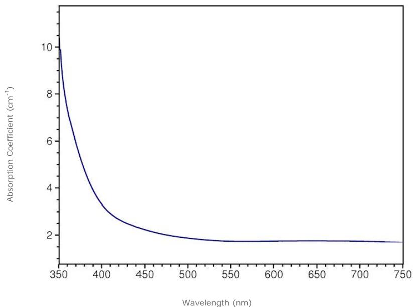
**Transmission absorption spectra** in the UV to near-IR range (250–1000 nm) were collected using a Hitachi U4001 spectrometer (2.0 nm slit, 1.0 nm data interval, and 120 nm/min scan speed). Unless otherwise noted, an unpolarized light beam was focused on the culet area of the optically unoriented sample.
