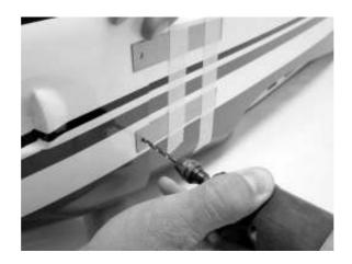
The engine bonnet is attached with four Allen screws as shown in the photos.
