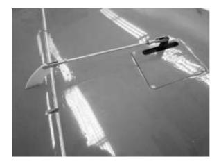
As shown in the photo, secure the hinges for the landing flaps using heat-shrink tubing.
