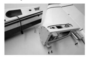
Use the  $\emptyset$  12 mm aluminium tube to put the horizontal stabiliser onto the fuselage to test the fit; the two extension cables must be routed through the openings of the horizontal stabiliser on the right and left.
