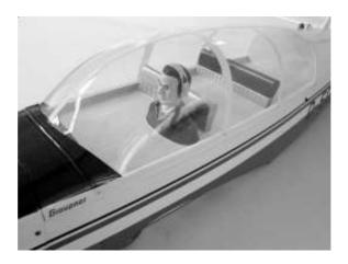
The cockpit canopy is attached to the frame using small pan-head self-tapping screws. A strip of tape all around has proven to be a good way to ensure that the cockpit canopy fits the frame uniformly.
