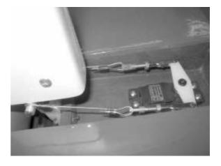
Here too, make sure that the nose gear is exactly in the neutral position when the servo is in the centre position. Later the nose gear steering servo and the rudder servo can be connected to the same receiver socket either using a Y-lead or via a mixer at the transmitter.
