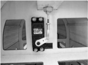
It is best to operate the aero-tow release mechanism using a momentary switch mounted on the joystick. The servo travel must be set accordingly.
