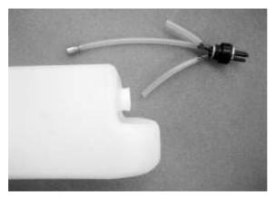
Connect a further length of fuel tubing to each stub tube projecting from the fuel tank. Mark the silicone tubes with a felt marker to show which of them runs to the motor, the overflow, and the filler.
