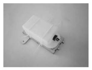
Push the fuel tank into the fuselage so that the three silicone tubes stick out through the drill hole in the bulkhead.
