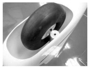
The wheels and wheel fairings must be aligned exactly parallel with the fuselage centreline.
