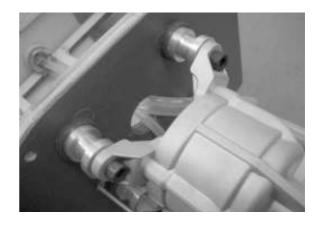
The throttle rod is adjusted so that the carburettor is half open when the servo is in centre position. The servo travel must be adjusted so that the engine stops when the throttle stick and trim are at the full back position.
