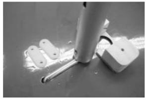
Drill pilot-holes in the wings for the retaining screws; then screw the tabs and the wheel fairing support block to the wing.
