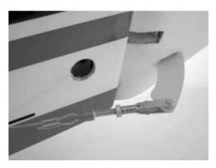
Then attach the rudder servo to the servo plate at the front of the fuselage.
