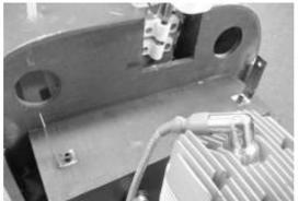
Now, the silencer can be attached to the aluminium brackets, and, together with the manifold, can be bolted to the engine; a drop of UHU thread-lock fluid should be applied to each bolt and nut to prevent them working loose.
