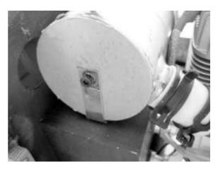
To fit the motor used, it is necessary to cut or file out openings in the engine bonnet for the silencer exhaust pipe, spark plug, et cetera. Position the engine bonnet on the fuselage in such a way that the clearance is about 2 mm between the spinner base plate and the front edge of the bonnet.
