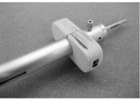
Fix the nose gear in the brackets by tightening the screw in the collet. Assemble the pull cables as shown in the photo.
