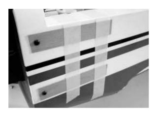
Unscrew the Allen screws, then push up the engine bonnet so that it moves under the strips and the spinner base plate is about 1.5-2 mm from the engine bonnet. In this position, mark the four attachment points on the engine bonnet.
