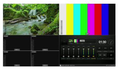
**PGM:** The Program window displays the on-air signal that's being recorded and/or broadcast. Set the Program signal by selecting one of the HDMI 1–4 PGM buttons.
