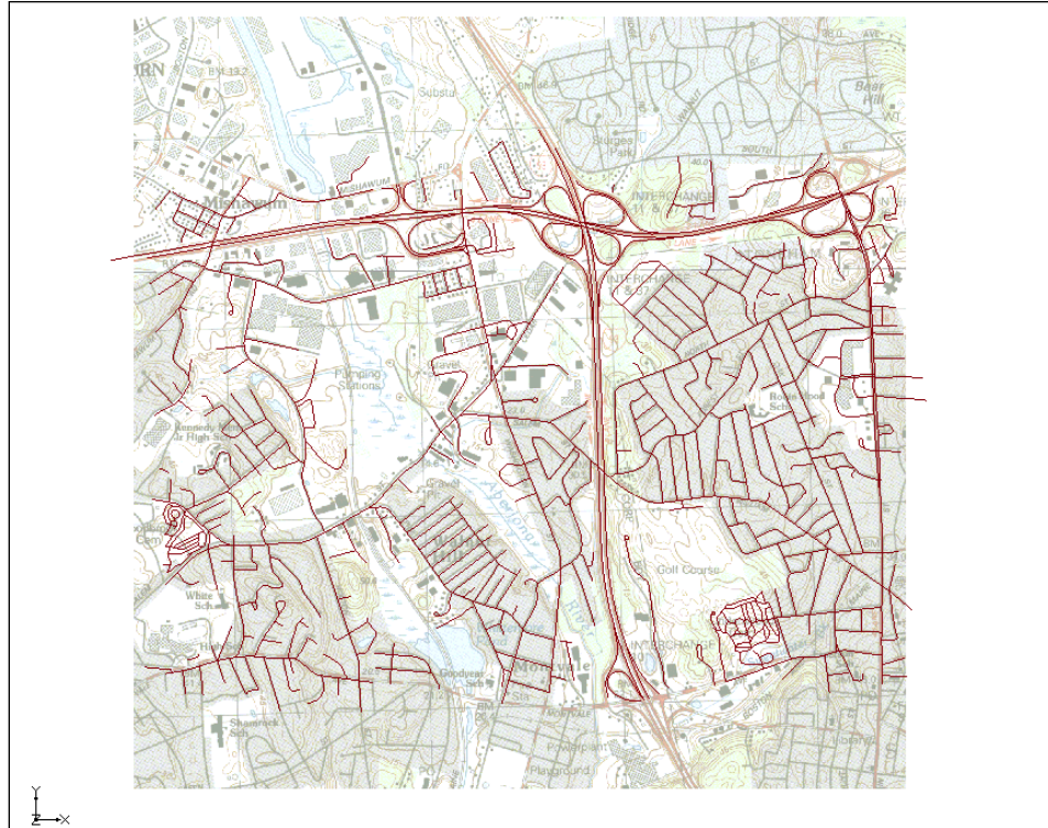
Figure 5 CAD data correctly positioned after specifying the projection
