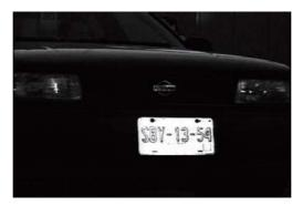
• **Plate Covered in Shadow:** Avoid placing the camera where it is subjected to direct sunlight, reflections or shadows, which may limit recognition performance.
