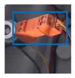
3. Then connect it to **External IR Wiring Pin** (see No. 2, *2.1 Internal Wiring*), as illustrated below.
