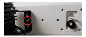
2. Thread all wires from GV-LIR32I8-070 through the node at the base of the supporting rack, and through the bottom of housing box.
