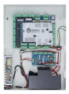
The GV-AS4111 Kit is a cabinet that includes a GV-AS4111 control panel, a power adapter board, a power supply and a backup battery case. The power supply powers the GV-AS4111 control panel as well as up to 8 output devices (12V, 0.5A per device).
