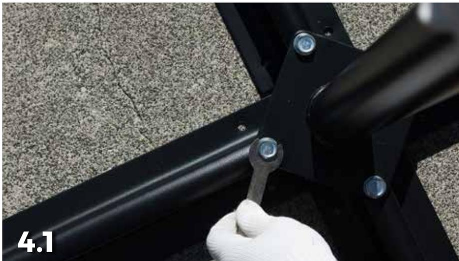
**TIP:** Try not over-tighten with the wrench.
