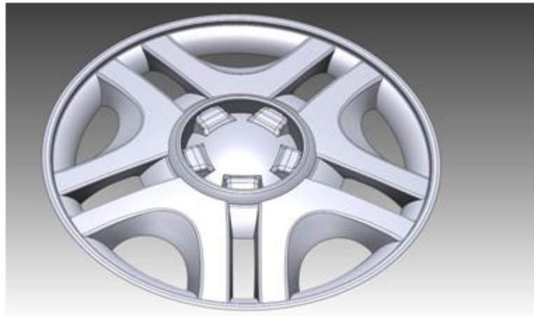
Figure 20: Creation of one entity and repeated circular pattern to create the entire object.
