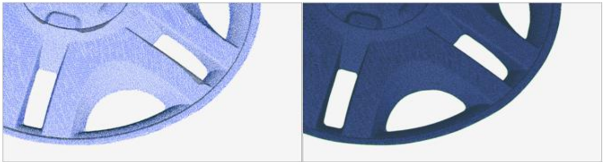
Figure 14: Point cloud vs. mesh file.
