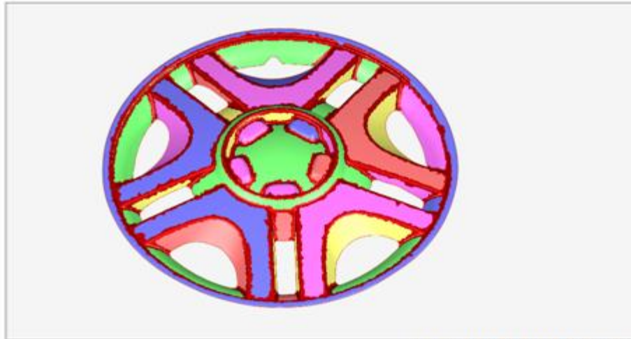
Figure 17: Representation of object into different regions/shapes (segmentation).
