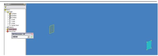
Then we make a sketch like the one below. Pay attention especially to the workplane, these have been dragged in the model browser so that is now under the sketch, and as a result can the geometry be projected. Also we give the dimension of projective centerpoint to the projective workplane. This dimension is a so called "driven dimension". Inventor indicates that his
