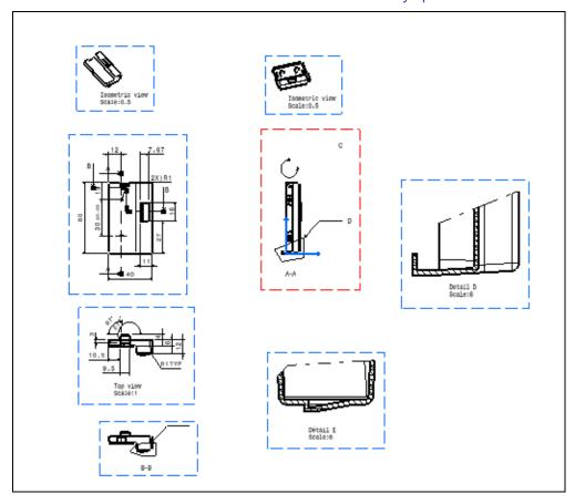
4. **Reposition** the detail view profiles and dimensions that have been moved.
