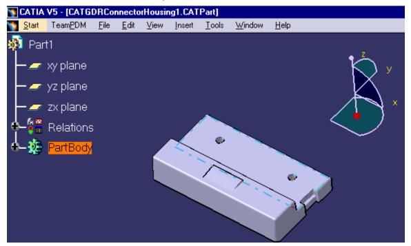
8. With the Dial (the view manipulator) **rotate** the isometric view in order to obtain a **view showing the inside** of the part.
