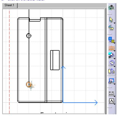
4. Double click **under the geometry** of the view to end the Offset section view profile
