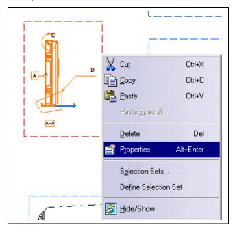
4. In the View Properties panel uncheck the Display View Frame option then click on OK.
