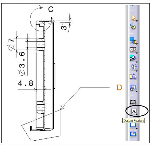
2. Select the **left edge** of the connector in the section view A-A.
