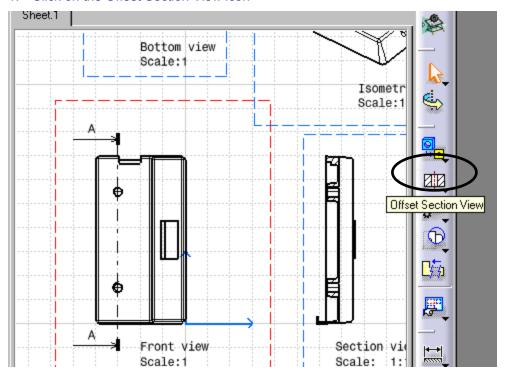
2. Build the following **Offset section view profile** with the same method described for the section view A-A. **Double click** to end the profile.
