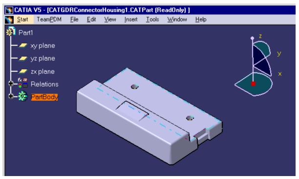
10. Use the **view manipulator** in order to have the view in the following configuration then **click** anywhere on the sheet to generate the views.
