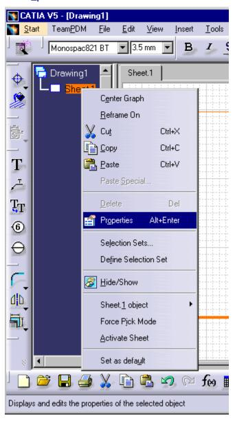
4. In the properties panel select Create projection views using first angle standard then click on OK
