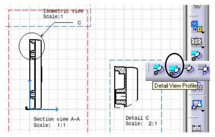
2. Build a **Detail View profile** around the **clip** of the Section View A-A
