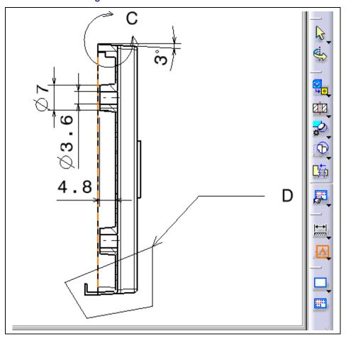
3. Position the Datum **outside the geometry**, then click on **OK** to accept the Datum feature.
