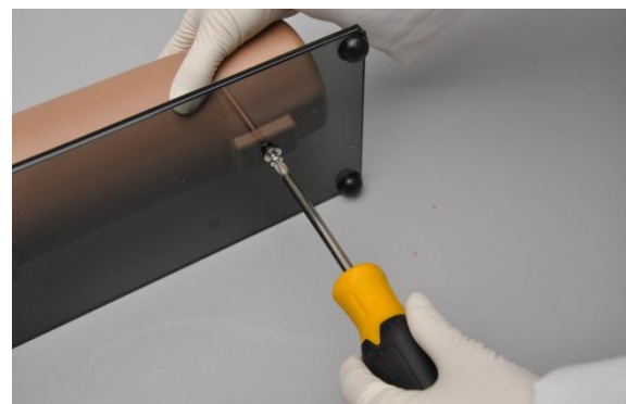
7. Reattach the left arm to the base using the screws and washes.
