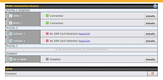
To disable a particular WAN connection, drag on the appropriate WAN by holding the left mouse button, move it the **Disabled** row, and drop it by releasing the mouse button.
