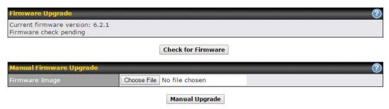
There are two ways to upgrade the unit. The first method is through an online download. The second method is to upload a firmware file manually.
