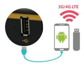
For increased WAN diversity, plug in a USB LTE modem as backup. Peplink routers are compatible with over 200 modem types.
