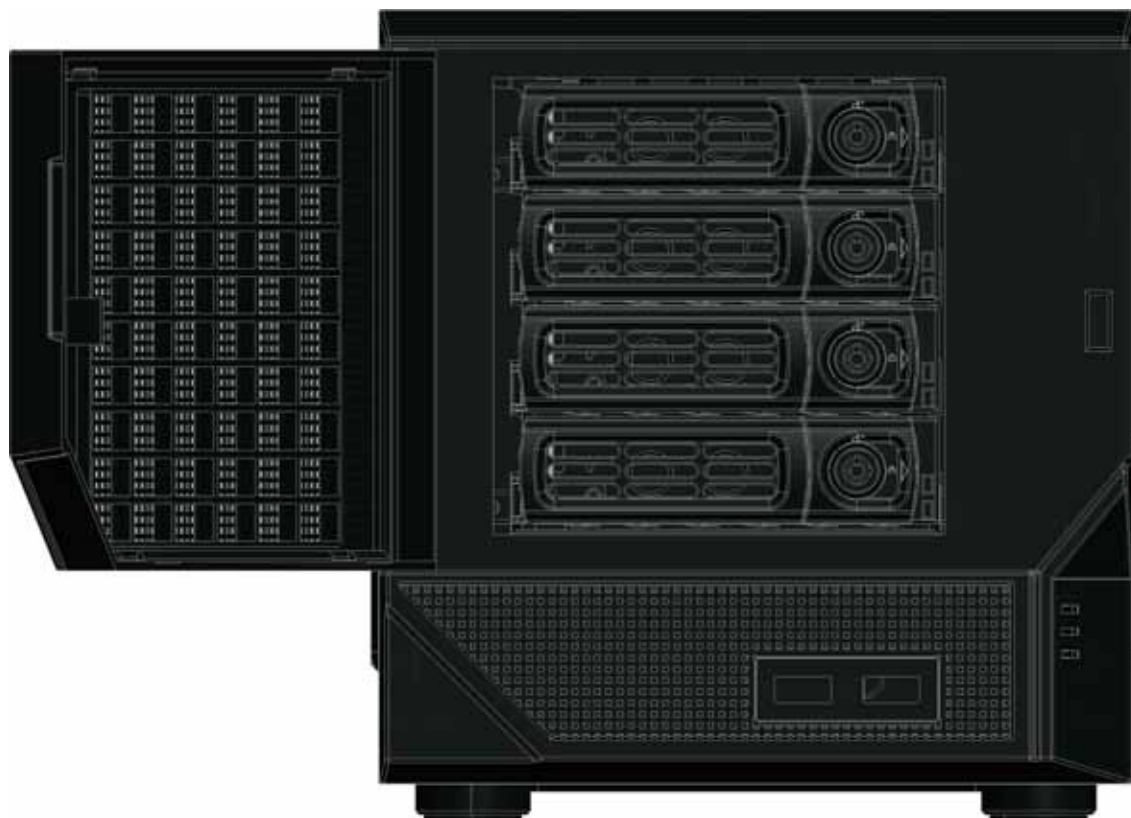
Figure 4: Hard disk bays on FortiRecorder 400D unit
