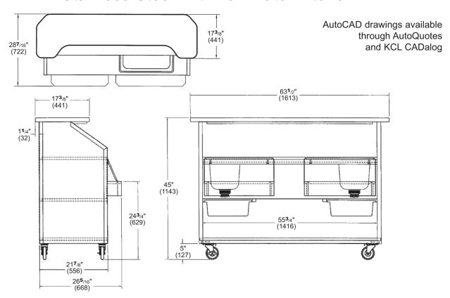
Dimensions: Overall Dimensions: 22-1/4" W x 63-1/2" L x 44-1/2" H (565mm W x 1588mm L x 1130mm H)
