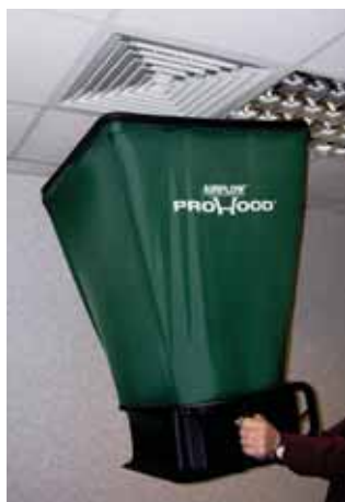
Figure 6.1 Balometer airflow measuring hood
