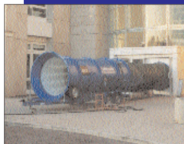
One of the BREFAN fans in position during the BRE pressure test at Barclaycard.
