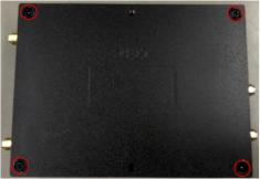
10. Complete by bringing both side panels to their designated location and assemble bottom cover with 4x Phillips chassis screws
