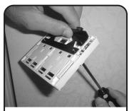
Alternately, the bracket can be assembled to the surface mount box before mounting to the furniture channel.
