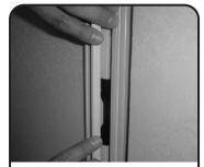
Raceway can be mounted to bracket with either adhesive and/or the two 6-32 x 1/4 inch screws provided.
