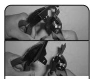
Prepare bracket for raceway mounting by breaking off the unused mounting hole section of bracket. The bracket will break cleanly and easily at the narrow joint by gripping both sides with pliers and bending back and forth 2 to 3 times as shown.
