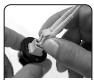
Insert the LC connector into the back of the Industrial outlet.
