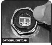
Place the panel nut over the flange and tighten to 1.69-2.26N-m (15-20 in-lbs).
