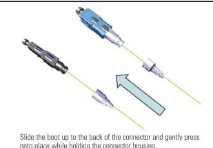
onto place while holding the connector housing.
