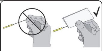
Clean the bare fiber with two passes of a 99% reagent grade isopropyl alcohol wipe, being careful not to touch the fiber after it is cleaned. Also be careful not to remove the reference mark.
