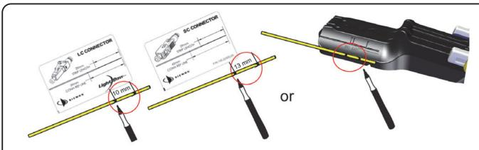
Locate the template card provided and follow the guide for the specific connector being terminated. The card depicts proper strip lengths for both SC and LC connectors. With the end of the fiber placed even with the end point shown on the template card, mark the strip length as shown. Also place the additional reference line mark indicated to be used as a visual aid during the insertion step.
