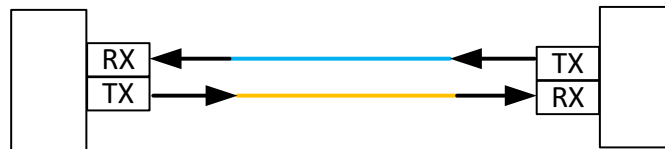
Figure 7-11: Duplex Transmission Polarity
