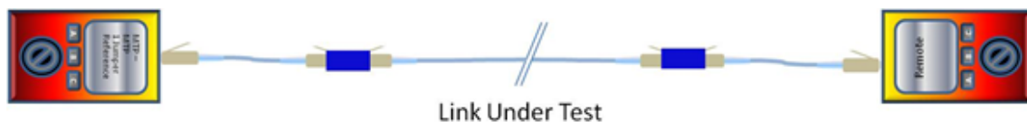
Figure 8-7: Optical Fiber Link Test
