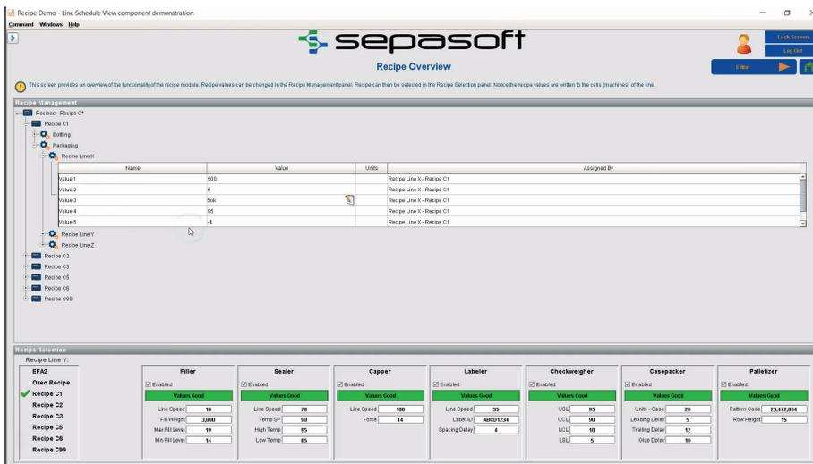
**Managing Machine Settings on a Large Scale** | Manage and quickly edit machine settings for a single machine, multiple production lines, and entire production areas.
