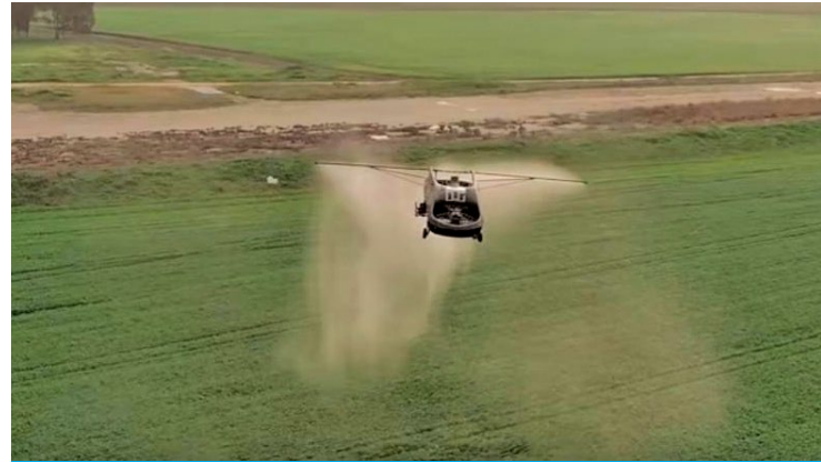
Ag-Cormorant, the high-payload, vertical-takeoff bi-rotor drone made by Tactical Robotics and Adama, represents the "future of aerial spraying," Adama's Senior VP of Strategy and Resources Dani Harari says.
