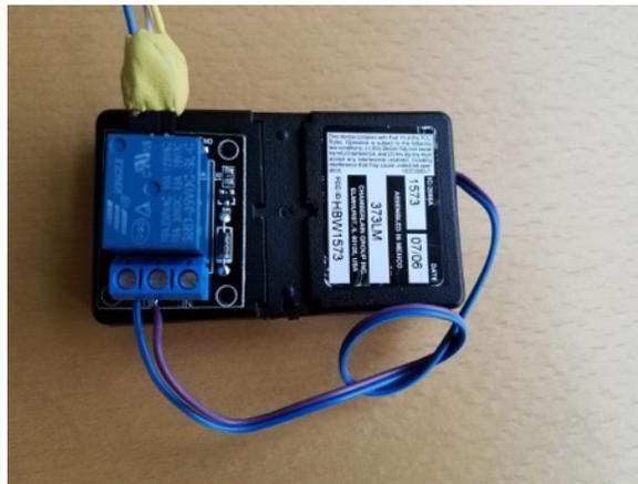
Back of remote with the case replaced, the relay module and wires attached.
