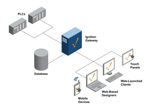
Ignition's most common architecture consists of a single on-premise Ignition Gateway connected to a SQL database, PLCs, and clients. In this case, all functionality is configured on the same Ignition Gateway. Ignition's licensing is unlimited. However, Ignition is limited by the size of the hardware. With more capable hardware, Ignition can handle more device connections, tags, and clients.
