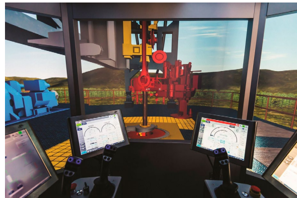
Drillmec created an innovative simulator for operator training.
