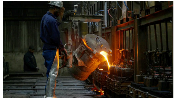
Ferroloy and Artek did not want to distract operators while they were pouring 2,700-degree molten iron.
