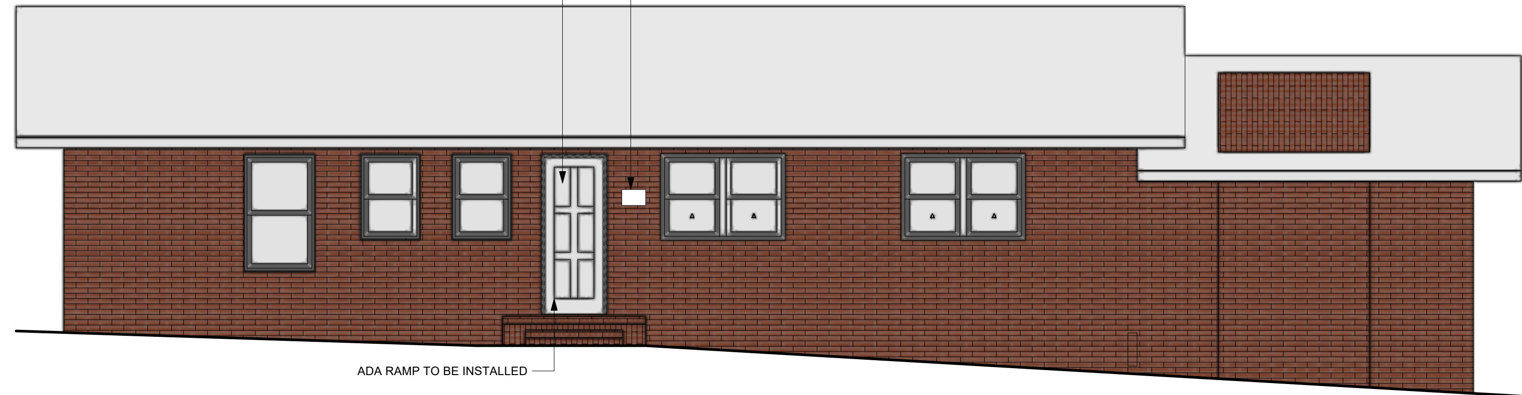
3 REAR ELEVATION (NORTH FACING) - EXISTING MATERIALS TO REMAIN; ACCESSIBILITY AND LIGHTING IMPROVEMENTS AS NOTED Scale: 1/4" = 1'-0"
